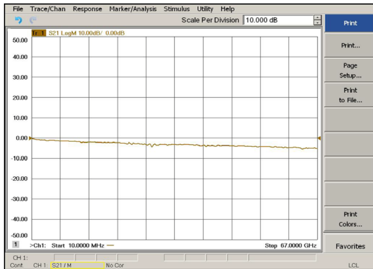
Figure 47 Source IN to Ports 5 to 8 Path Response
