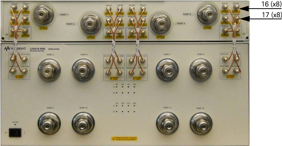
Figure 10 12-Port Interface Connections
