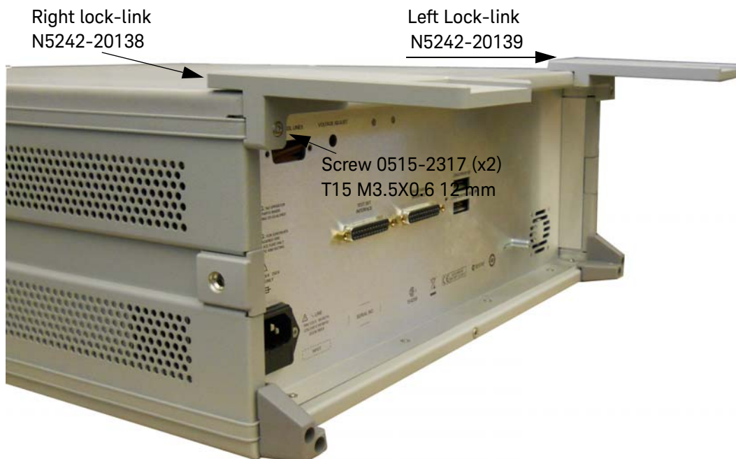
Figure 7 Install Lock-links to the Test Set
